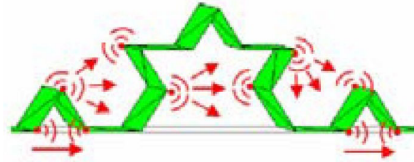
Figure 5. Signal coupling at angles in Koch curve fractal
